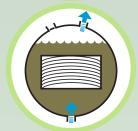
Cylinder is flooded under vacuum with Tanalith E wood preservative, with Tanalith Extra or Tanatone additives, if required.
