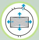
Timber is loaded into treatment vessel. Initial vacuum is applied - timber cells evacuated of air. Vacuum held.
